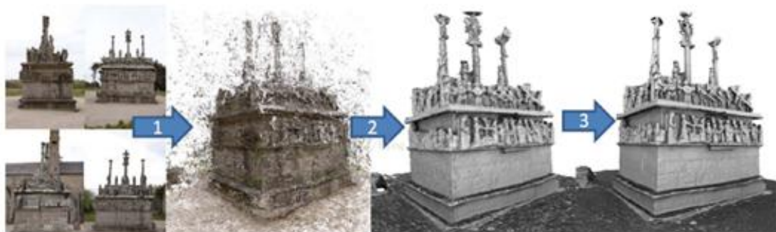
Fig. 1. Reconstruction pipeline. 1) Generate a points cloud. 2) Extract a visibility-consistency mesh. 3) Refine the mesh with photo-consistency optimization and regularization.
